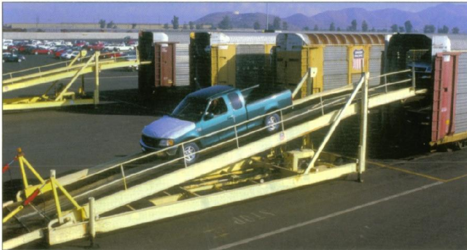
Railroads transport 70% of all cars and trucks sold in the United States. This new pickup truck is being unloaded from a bi-level (double-deck) Union Pacific autorack car at a distribution center in California. Autoracks also come in tri-level configuration. (Chuck Fox photo)
