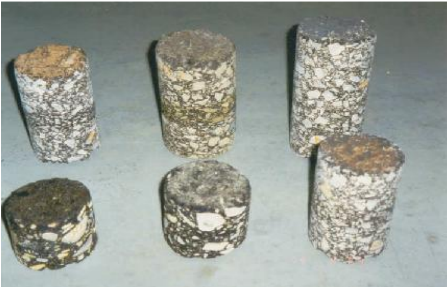
Dense-Graded Highway Base Mix 1 – 1 ½ in. Maximum Size Aggregate Asphalt Binder +0.5% above Optimum Low to Medium Modulus Mix, 1 - 3% Air Voids
